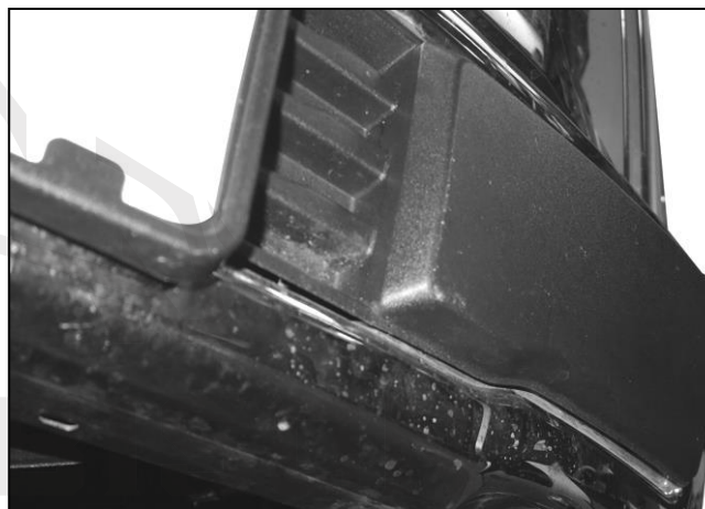
(Fig 5) Remove bumper pads to access splash guard hardware if necessary. 2017 F150 pictured
