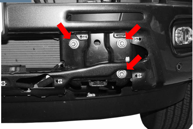
(Fig 6) Remove the nuts attaching the bumper to the frame and remove the bumper
