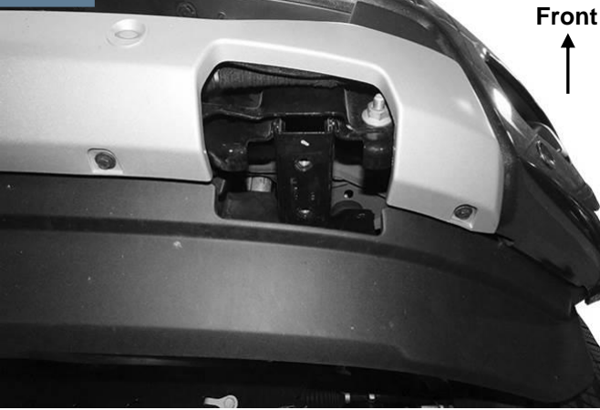
(Fig 2) Plastic cover and tow hook removed
