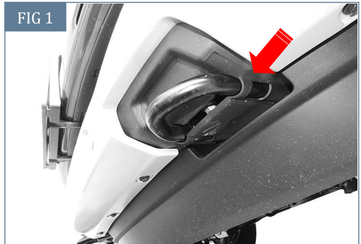
(Fig 1) Remove plastic covers and tow hooks
