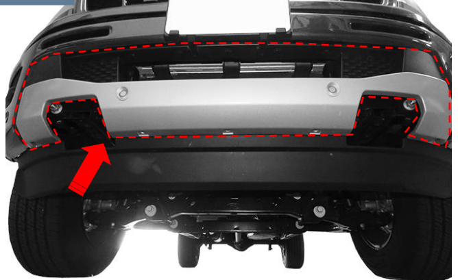
(Fig 4) Remove the center plastic cover
