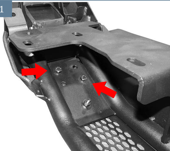
(Fig 11) Attach Wing to Bumper (driver/left side illustrated)
