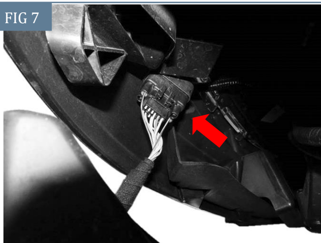
(Fig 7) Pull the bumper out slightly and unplug the outer wire harness
