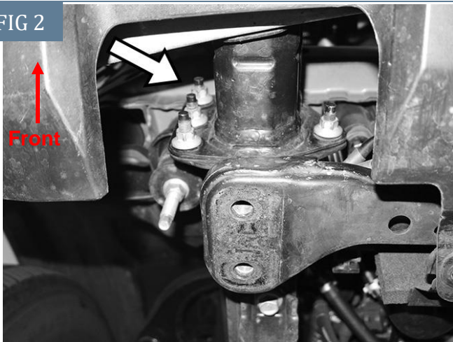
(Fig 2) Locate the (3) outer hex nuts attaching the original bumper bracket to the frame. Reuse the center and top hex nut to attach the Top Frame Bracket to the front of the bumper bracket
