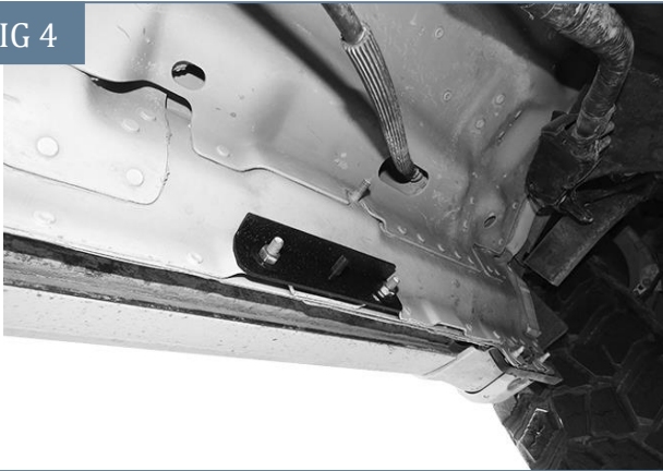
(Fig 4) Example of the Support Bracket (#1) attached to the threaded studs
