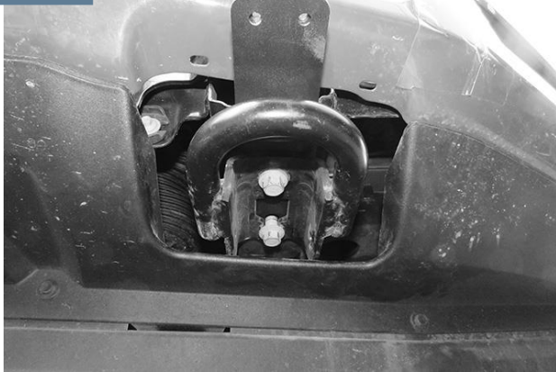
(Fig 16) Support Bracket installed between tow hook and bottom of frame
