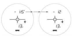
The upper part of LCD shows the angle of uphill / downhill then change to the horizontal distance that is the true distance.
