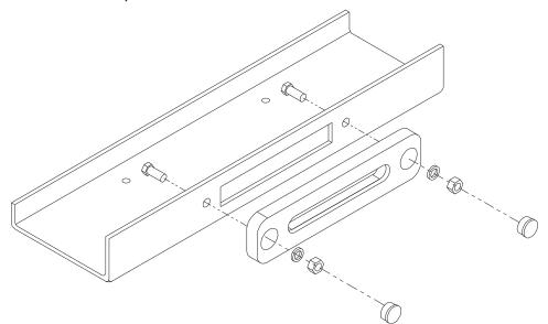
• Attach the winch to the plate with capsrews, lockwashers and nuts (not included).
