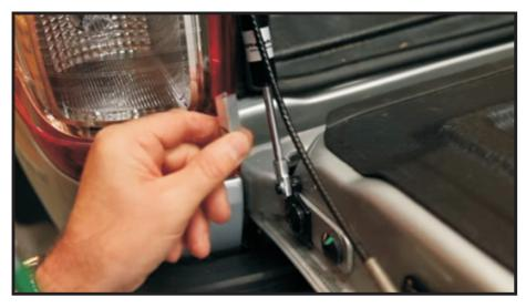
The spacer should not be removed before installation is finished.
