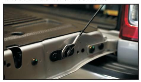
Temporarily remove the cable from the tailgate.
