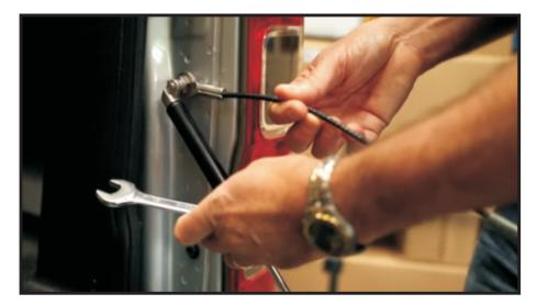
Place the strut to the body with cable attached.
