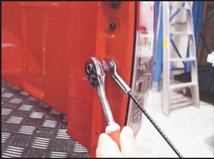
1. Remove the bolt of the cable from your tub.
