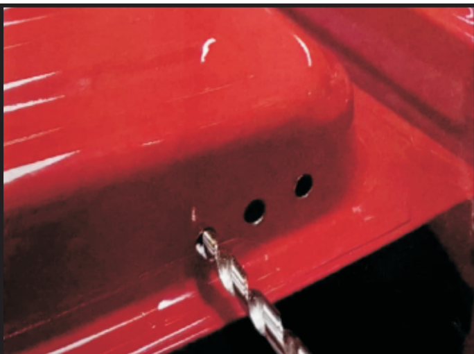
5. Drill the three holes to 10mm. TIP: drill smaller holes first to locate the bit.
