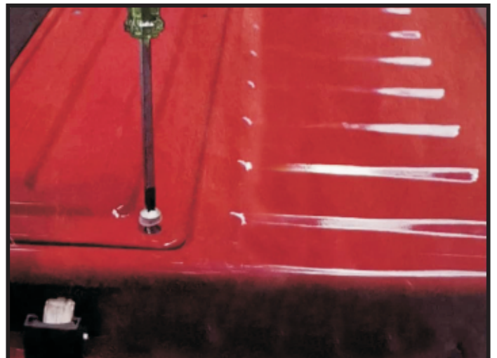
6. Remove the access panel of the tailgate.
