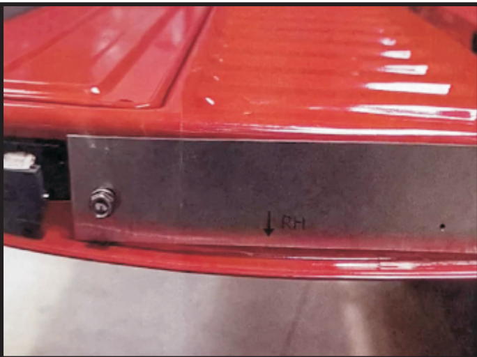
3. Bolt on the drilling template as shown.
