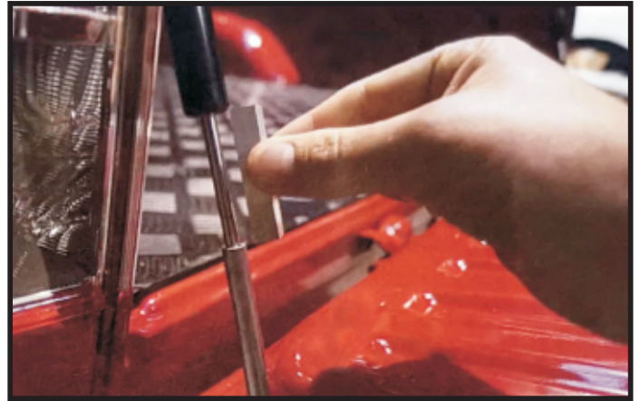
14. Repeat the same process on the passenger side for up strut and remove the spacer once installed.
