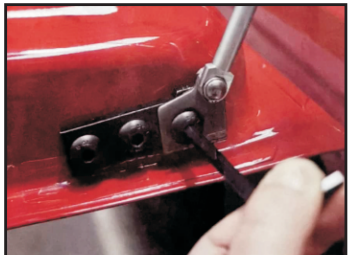
12: Place the bottom of the strut over the tailgate bracket and then screw in the third bolt.
