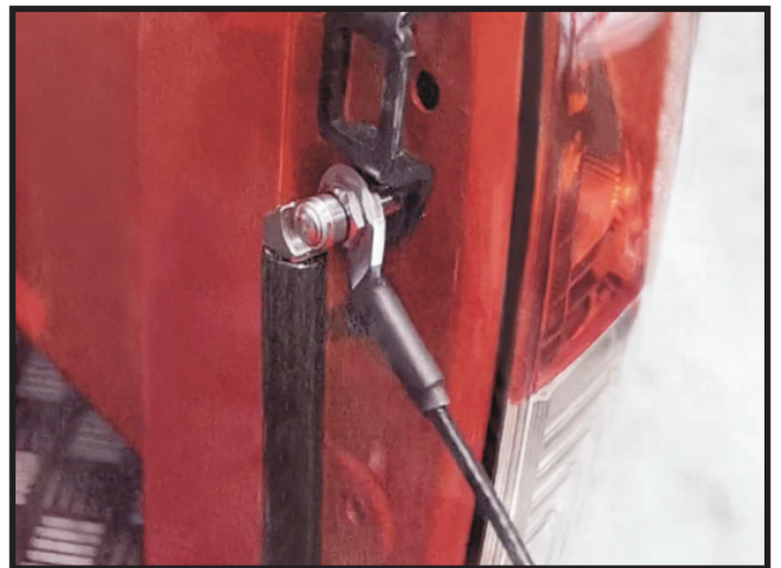
10. Install the strut and new cable supplied.
