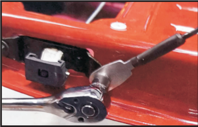
13. Reinstall the removed cable bolt in step 2 and place the cable on first.
