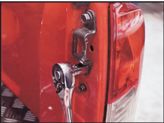
9. Remove the lower striker bolt from the tub.
