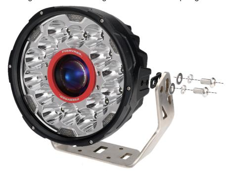
3. When mounting to the desired application, the order of the hardware is as follows: Bolt > Mounting Bracket> Rubber Pad> Mounting Platform> Washer> Spring Washer> Nut.
