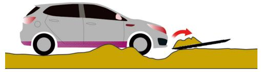
3. Create a gently sloping formation in the soft ground of the direction the vehicle is intended to travel. Place the tracks hard against the tyres as shown in the diagram to make it easy for the tyres to be able to engage the teeth.
