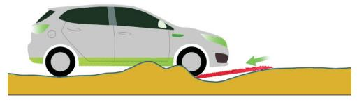
4. Shift into your lowest gear and move slowly and carefully onto the tracks. Avoid wheelspin when on the tracks. Slowly accelerate to gain vehicle momentum before leaving the tracks and entering onto a more stable road surface.
