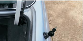
Install and tighten the rubber antenna 4.
