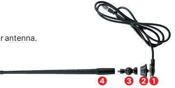
Insert the bolt of 1 through the mounting hole from the inside. Then install and tighten 2 and 3 onto the bolt.
