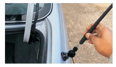
Connect the antenna plug with plug from the vehicle.
