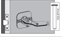
6.Routing the cable and connector through cable hole on interior assembly.
