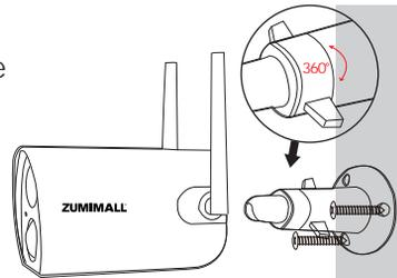
Rotate the button counterclockwise to take off the camera.
