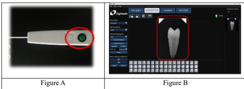
7. Checks the image quality, if it is not good, adjust the X-ray transmitter parameters(refer to chapter 7), repeat step 5-6.
