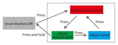
(Drum machine operation diagram)
