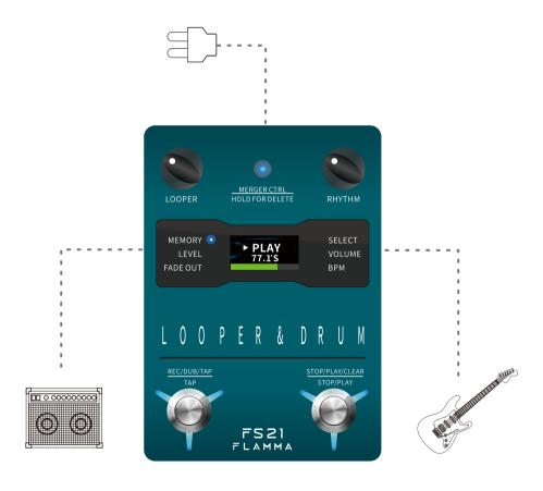
FS21 has both LOOPER and RHYTHM modules. Users can switch between LOOPER and RHYTHM by pressing both footswitches simultaneously. The LED of LOOPER (blue) and RHYTHM (red) will indicate current module.
