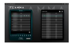
**Name:** List on the left-hand side shows 40 save slots in MEMORY. Slot name in dark indicates the looper file and its duration. Slot name in grey indicates empty slot.
