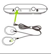
4.2.4 Grab the corner of the electrode pad and peel it off the protective film, and **do not pull the wire directly.** Attach one pair of electrode pads to the massage area and press the edge of the electrode pads firmly on your skin to make sure full contact. Use the second port with two additional pads on other pain areas for relief. (Make sure the unit is off when you attach the pads.)
