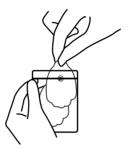
4.2.3 Connect one pair of electrode pads to one lead wire and connect the other end of the wire to the A or B output of the device.
