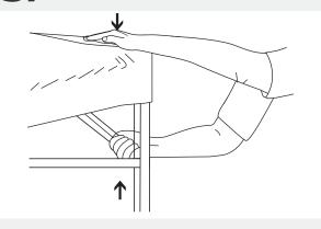
Push the leg release button and pull down the leg to extend each leg to the desired height
