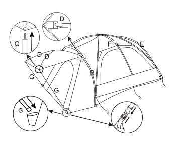
Step 5: Install the two Pole D (Labeled White), forming the X of the front roof. Install Pole G (Steel Poles), as follows.
