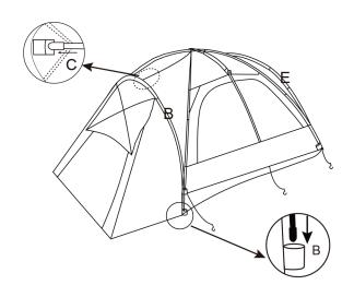
Step 4: Install Pole C (Labeled Black) inside the roof of the tent.
