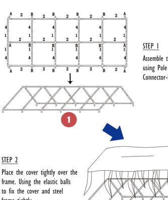
Assemble the upper frame and the roof frame using Pole #1, #2, #4 & the Connector-A, Connector-B.
