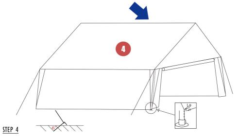
Hang the side panels to the holes by the Elastic Balls. All side panels can be hung or took down separately. Pull the leg cover tight by the elastic ball and attach the metal hooks into the tube holes near the feet. If the cover becomes loose, tighten by moving the hook to a lower hole. Then secure the tent with Ropes and the Stakes. We recommend the Stakes are at a 45 degree angle in the ground facing away the tent to ensure maximum tension.
