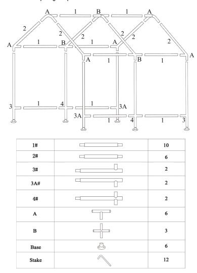
Assemble the greenhouse with all the parts above.
