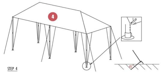
Pull the leg covers tight and attach the metal hooks into the tube holes near the feet. If the cover becomes loose, tighten by moving the hook to a lower hole. Then secure the tent with Ropes and the Stakes. We recommend the stakes are at a <u>45 degree</u> angle into the ground facing away the tent to ensure maximum tension.
