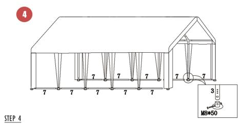
Connect all leg poles on the ground using Pole #7 and fixed it with a bolt.
