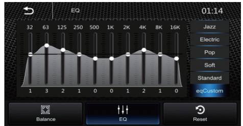
10-Band Equalizer 10 band of EQ tuning, slide the EQ bar to tune each band frequency level according to user preference. Touch Reset to set all Band to 0.
