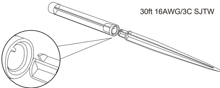
2. Insert the stake into the ground. Keep out of high traffic areas to prevent tripping.
