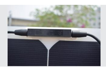
Each panel comes with MC4 male and female connectors that can connect easily to solar compatible devices. Connection cables are device-specific. The Junction box has IP67 protection.
