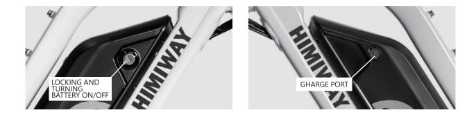
Always charge your battery in temperatures between 10 and 26 degrees Celsius and ensure the battery and charger are not damaged before initiating charge. If you notice anything unusual while charging, please discontinue charging and use of the bike and contact Himiway Bike for help.
