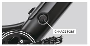
Always charge your battery in temperatures between 10 and 26 degrees Celsius and ensure the battery and charger are not damaged before initiating charge. If you notice anything unusual while charging, please discontinue charging and use of the bike and contact Himiway Bike for help.
