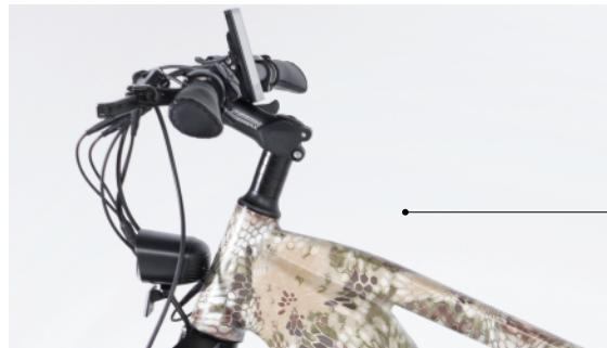
**NOTICE:** In addition to angle, the height of the handlebar can be adjusted by adding or removing the headset spacers if needed. For those without experience, we recommend having a professional make such adjustments for safety reasons.
