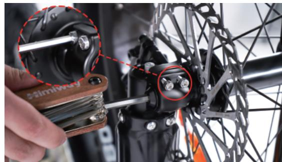
**WARNING:** Do not pull the brake lever without having either the red pad or the brake disc inserted, as this will damage the hydraulic brake caliper.
