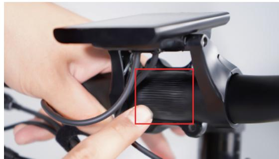
**Step 3:** Tighten bolts to handlebar stem, but don't tighten completely as you may want to further adjust the angle later to align more precisely. Test the positioning, and adjust the handlebar to your preferred angle. After determining the best position, completely tighten all the bolts on the stem.
