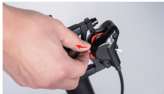
**Step 5:** Align the fork dropouts with the axle of the wheel hub, making sure the dropouts are fully seated on the axle. Also ensure the brake rotor is properly inserted into the caliper.
