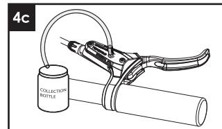
Step 8: Start filling the brake with new mineral oil by slowly pushing the syringe. Air bubbles may come out of the reservoir. Continue pushing fluid until you no longer see bubbles coming out of the tube .(See 4d)
