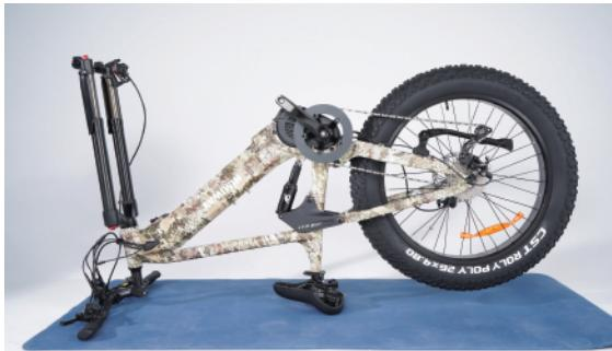
**Step 2:** Remove the plastic axle guards from the front wheel, being careful to avoid contact with the brake rotor set.
