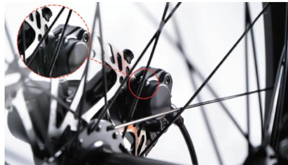
**Step 6:** Reinsert the hub axle in the same direction as before. Then reinsert the bolt into the hub axle and tighten, also tighten the two nearby bolts securing the bracket as shown in the image.
