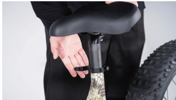
**WARNING:** Overextending the seatpost can cause it to break or come off your bike, putting you at very high risk of serious injury or death. Avoid this danger by inserting your seatpost into the seat tube far enough that the minimum insertion point is no longer visible.
