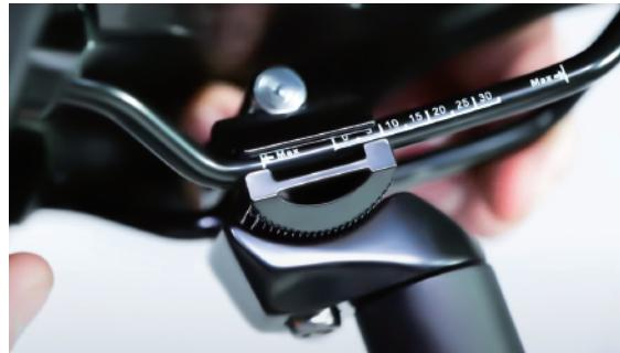
**NOTICE:** The seat angle has been preadjusted to factory safety standards. Please make note of original settings, and only adjust if necessary.
