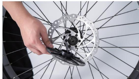
**Step 3:** Loosen the two small bolts securing the bracket around the hub axle, as shown in image A. Then, remove the side bolt in image B
