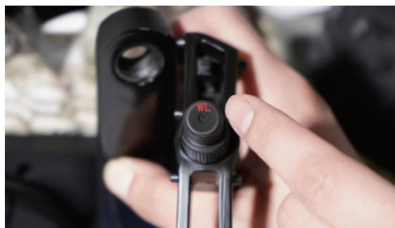
Before you install the pedals, apply a small amount of waterproof grease onto the spindle. Start threading the pedal on by hand to ensure the pedal is going in perfectly straight, rotating in the direction of the pointer shown on the crank. If it is not spinning smoothly, make doubly sure that you have the correct left or right pedal. After initial hand-tightening, finish tightening the pedals with a standard 15mm wrench .
