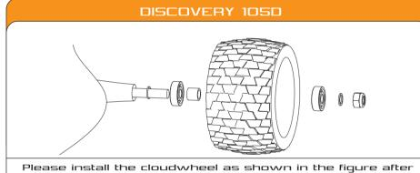
the sleeves must be installed.
