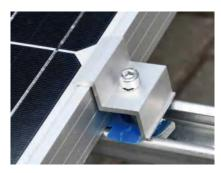
Use the clamps in package to set panels on the whole bracket, double-head middle clamp to put in the middle of two panels, the one side clamp to fix one panel's side. Use the hexagonal screwdriver to make them tightened
