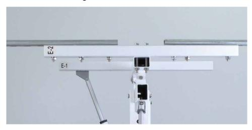
Put on the cross rods G-3 and G-4 on E-2 rod with M10\*60 screws(for firmly holding the panels, the screw should be put into the second hole of G-1, G-2 rod). Same way to fix G-1, G-2 rods on E-1 rod
