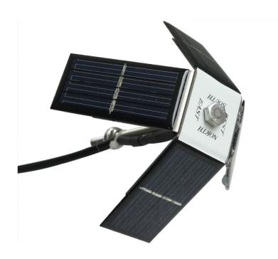
The detection head is a unique four-quadrant silicon crystal type, which generates four different solar radiation voltages in four directions and transmits them to the motherboard via 5-core cable. The installation method is M6 bolt fixation. All parts are made of aluminum and stainless steel. The silicon crystal plate is made of solar glue board production process, and the back welding line is covered with waterproof silica gel, which can meet the service life of ten years.
