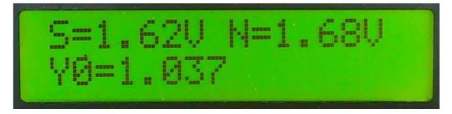
5. This page means to display the voltage output value of the south/north of the azimuth detection head and calculate its corresponding ratio Y0. It is used as a reference. It cannot be adjusted. Press  $\downarrow / \uparrow$  to turn the page and it will go to the next page:
