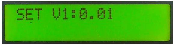
8. Set V1 value, which means the tracking accuracy value. It means that when the difference in the solar radiation voltage between the east and west and the south and north of the azimuth detection head is lower than this value, it is deemed to align with the sun; otherwise, it is not aligned and needs to drive the platform action to align. The minimum value can be set to 0. Key  $\rightarrow/\leftarrow$  can realize the addition and subtraction of parameters.
