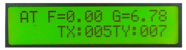
• In this state, the controller will compare the voltage values of the azimuth detection head east and west as well as south and north, and control the platform. When an axis is aligned, the TX/TY intermittent waiting time will be entered. After the time countdown is over, repeat the comparison and control. To implement the platform tracking process.
