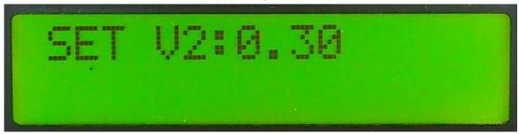
7. Set V2 value, V2 means the threshold value of wind speed exceeding the limit. It means that when the signal voltage value output by the wind speed sensor exceeds V3, the current wind speed is considered to be a threat to the platform, and the controller needs to perform protection action on the platform. Key  $\rightarrow/\leftarrow$  can realize the addition and subtraction of parameters.
