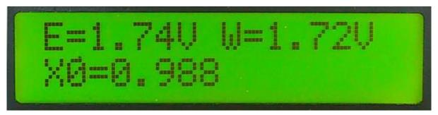
4. This page means to display the east/west voltage output value of the azimuth detection head, and calculate its corresponding ratio X0, is for reference, can not be adjusted, press " \ / \ " to turn the page, will enter the next page:
