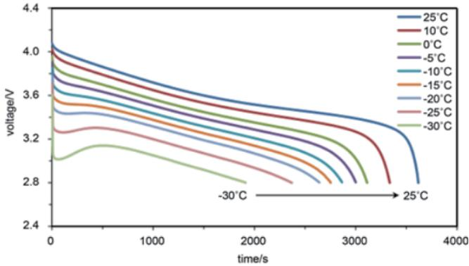
Lithium batteries rely on chemical reactions to work, and the cold can slow and even stop those reactions from occurring. Unfortunately, charging them in low temperatures is not as effective as doing so under normal weather conditions because the ions that provide the charge do not move properly in the cold weather.
