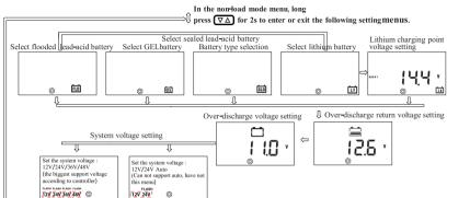
Battery Types, Charging Voltages (Lithium Battery), Over-Discharge Return and Over-Discharge Voltage Settings
