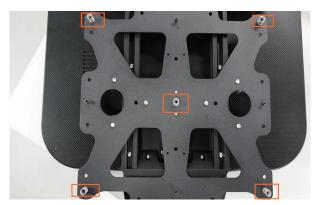
2. Tighten the screw at the center of the aluminum base plate close to but not over its maximum torque. Unscrew it about 6~7 circles. Check if the screw on the aluminum base plate has been put in place tightly enough.
