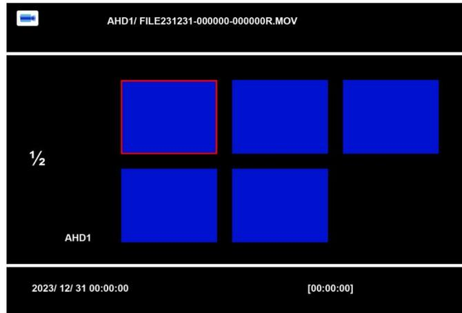
You can switch to the AHD1 or AHD2 video playback panel by pressing the **V1/V2** button.
