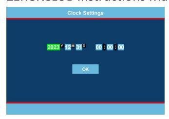
Press  $\mathbf{M} \to \mathbf{Go}$  into the **Clock Settings**  $\to$  **MODE**  $\to$  +I- (Increase time/ decrease time)  $\to$  **MODE** (confirm and go to the next date/time settings)
