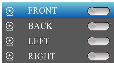
Front/Back/Left/Right each represent the camera's image of CAM1/CAM2/CAM3/CAM4 (FRONT=CAM1, BACK=CAM2, LEFT=CAM3, RIGHT=CAM4)
