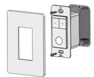
Note: Do not over tighten the screws, as it could restrict the operation of the switch.
