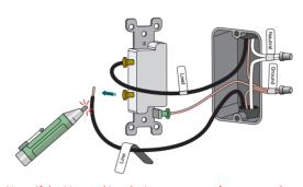
Note: If the Line and Load wires are reversely connected, the switch will not work.
