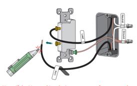
Note: If the Line and Load wires are reversely connected, the switch will not work.
