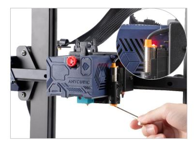
3. Return to main menu, click **Prepare**  $\rightarrow$  **Leveling**  $\rightarrow$  **Auto-leveling**  $\rightarrow$  **OK** on the pop-up interface. The print head and heated bed will be heated up first, then the print head will probe the spots on the platform automatically. This will take a few minutes, please be patient.
