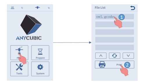
\* Before printing, the nozzle will start heating after the heated bed reaches target temperature. When the temperature reaches target value, the printer will start printing.
