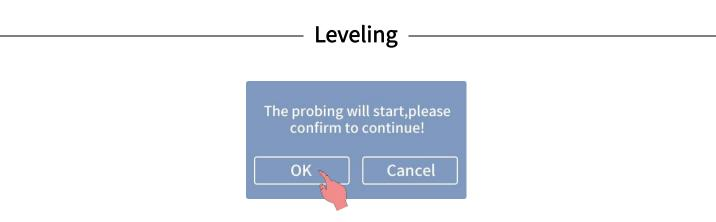
4. After probing the platform, put a piece of paper onto the platform, click **Z offse**t  $\rightarrow$  + or — to adjust the Z-axis height until the nozzle touches the paper (feel slight drag resistance when pull the paper), then click **OK**.
