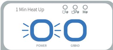
Insert the Power Plug. Press POWER BUTTON, LIGHT pulses = heating up. GRINDER LIGHT fully illuminated = Grinder ready to use.
