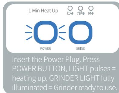
Insert the Power Plug. Press POWER BUTTON, LIGHT pulses = heating up. GRINDER LIGHT fully illuminated = Grinder ready to use.
