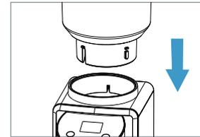
(15) Assemble the bean hopper ⑥ by match the white arrow with the white lock mark in the ring and rotate.
