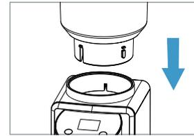
(1) Assemble the bean hopper ⑥ by match the white arrow “ ▼ ” with the white lock “ 🔒 ” mark in the ring. Rotate the bean hopper ⑥ clockwise to lock it and the grind size ring setting ⑨ can be adjusted.
