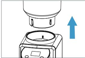
(8) Disassemble the bean hopper ⑥ . Take the brush ⑭ from the hopper lid ⑤ .
