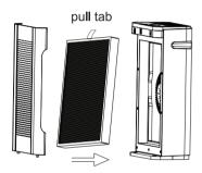
**NOTE:** If the front or back shell are not installed properly, it will remain power off.
