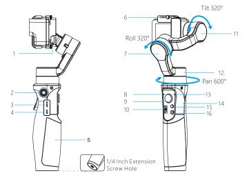
1.Mini USB DC out Port 2.1/4 Inch Extension Screw Hole 3.Trigger Button 4.USB DC Out / DC In
