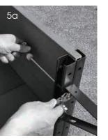
Use a 5mm hex wrench to hold the bolt and a 13mm wrench to tighten the nylon lock nut.
