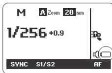
If the battery power is low,
